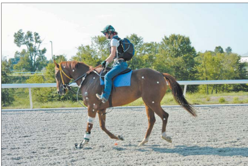
Hoof accelerations, ground reaction forces and horse speed were measured on dirt (top photo), turf (middle photo) and synthetic (bottom photo) surfaces at the Keeneland Race Course in Lexington, Kentucky. Instrumented horses were walked, trotted and cantered through the data collection corridor during three to four trials each of trot and canter.
